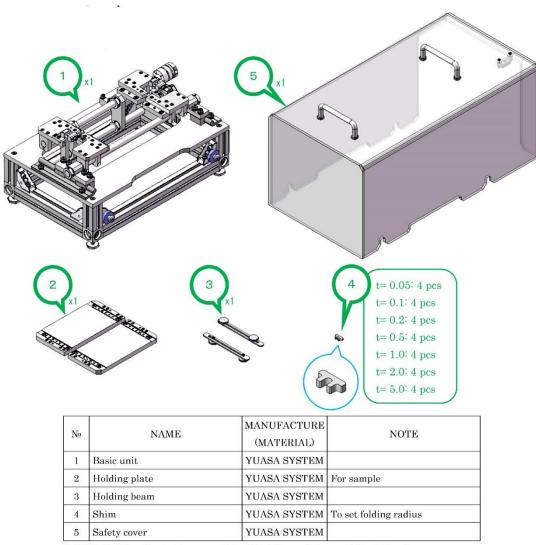
NOTE The Cartridge consist of holding-plates and holding-beams.
