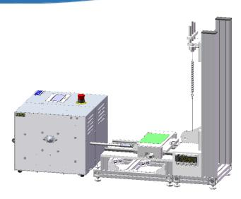
The optional load-cell attachment with other non-contact sensor components can in addition, detect and replicate testing conditions for material sagging.
