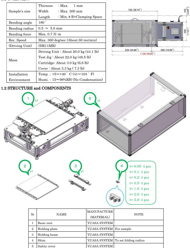
NOTE The Cartridge consist of holding-plates and holding-beams.
