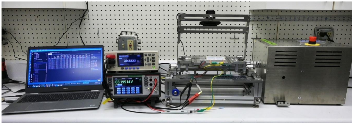
Figure 1. Flexdata Experiment Using a PC Laptop, Hioki Resistance Meter, Keithley Digital Multimeter, Yuasa Clamshell Test Jig with Logitech Camera Mounted on a Bridge, and a Yuasa DMLHP Motor Drive Unit
